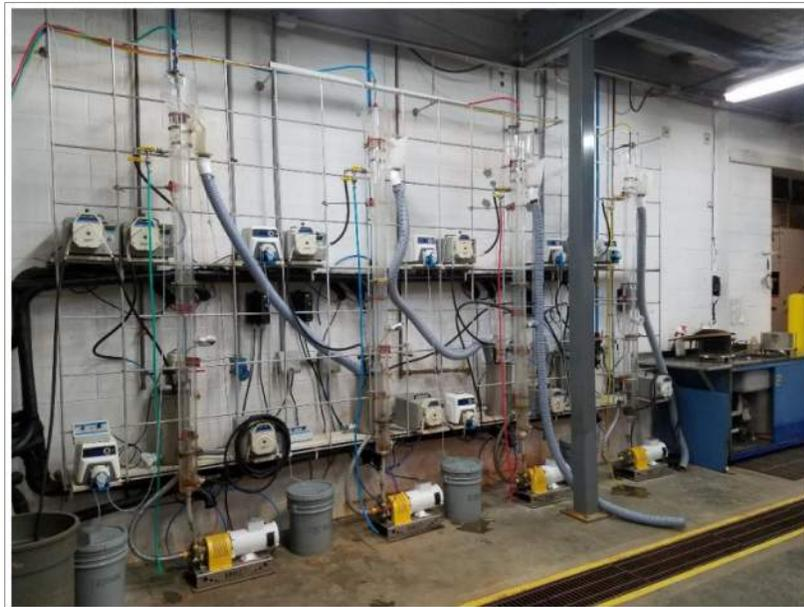
Table 13.14, below, details the mass balanced circuit results ascertained during continuous operation of the rougher-cleaner-cleaner-scavenger column flotation circuit. Final circuit P<sub>2</sub>O<sub>5</sub> recoveries and grades varied, as a result of variations in feed size distribution, head grade, and operating parameters.
