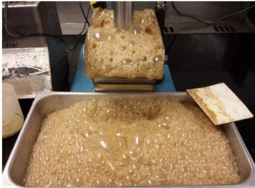
Figure 13.7 illustrates the impact of the cleaner stages of concentration; of significance is the color of the rougher tails (on the left) and the third cleaner concentrate (on right).
