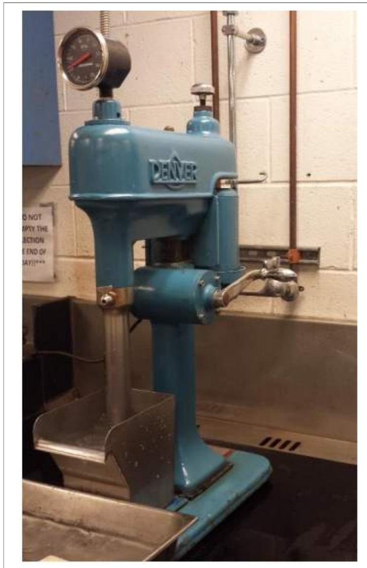
The following photos show the rougher flotation of fresh amphibolites (MAMP) and saprolite of amphibolites (AMPSAP), respectively.
