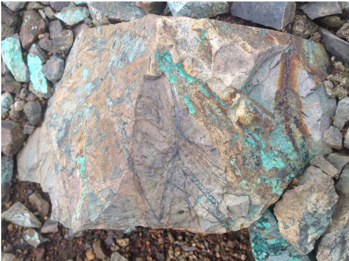
Figure 3. Example of copper mineralisation at surface on the Canhada Target. Hydrothermally altered volcanic rock with malachite filling fractures in stockwork pattern. Sample grading 4.09% Cu.
