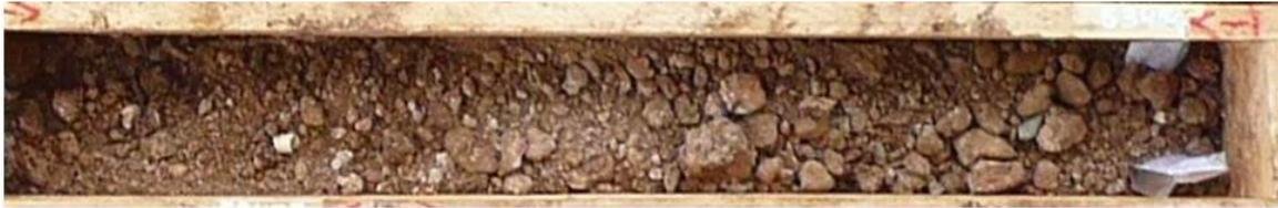
Oxidized meta-carbonatite, yellowish brown, with quartz veins and P2O5 high grade (>20% P2O5, up to 32% in rock). Biotite, KF and chalcedony veins occurs. Magnetite and hematite occur disseminated in the meta-carbonatite.
