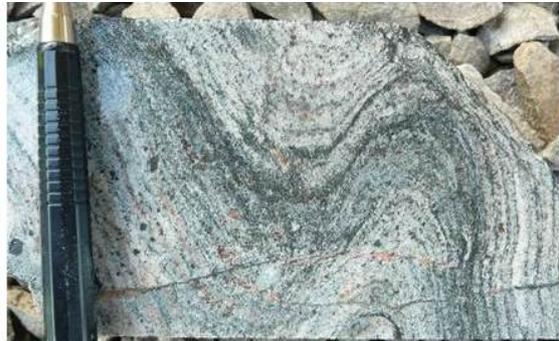
Fresh calcitic meta-carbonatite, white to pink. Occurs foliated and folded, metamorphised in amphibolite facies. Magnetite crystals occurs disseminated and strings of sulphides are common. Average P2O5 values of 5.00% P2O5 and up to 12.90% P2O5 (TED-11-016).
