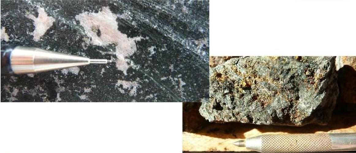
Dark green amphibolite. Recrystallized and few deformed. Fresh amphibolite returned average P<sub>2</sub>O<sub>5</sub> values of 2.29% P<sub>2</sub>O<sub>5</sub> and values up to 7.29% P<sub>2</sub>O<sub>5</sub> (TED-11-007). Amphibolite saprolite returned average grade 3.99% P<sub>2</sub>O<sub>5</sub> and values up to 9.96% P<sub>2</sub>O<sub>5</sub> (TED-11-002).
