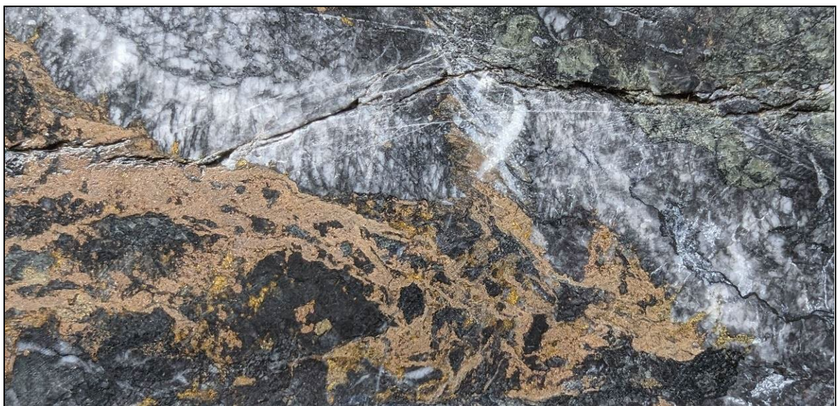
(Photo 3) In this example, chalcopyrite (2% approx.) postdates and replaces previous larger patchy sphalerite (light brown) replacements (between 10-20%), mainly hosted in a dark breccia zone where both sphalerite and chalcopyrite show similar "flame" like replacement textural appearance, and both may have used the same pathways from the same base metal source and deposition paths (SB14-02 , detail from interval 20.0m to 21.0m). For assay results refer to Table 3.
