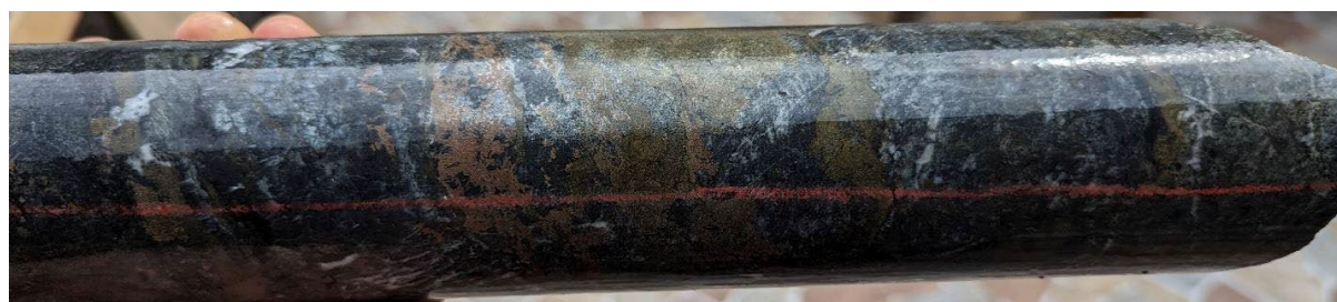
(Photo 7) SB14 04 (dark breccia, pyrite and sphalerite replacements). Recent assays returned 0.21 gpt Au, 9065ppm ((0.91%) Zn, 1.78 gpt Ag over 0.60* meters (From 11.7m to 12.3m).
