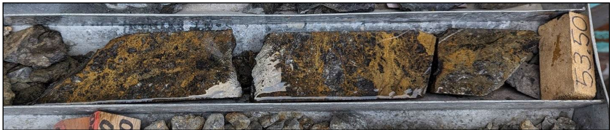
(Photo 4) Chalcopyrite is the almost dominant sulphide in this high-grade (50% cpy approx.) zone. It presents a unique “flame” like and semi-massive texture paralleling the deformation and strain directions of the host shear zones in a dark breccia host rock (D13-07 from 53.0 to 53.5). For assay results refer to Table 3.
