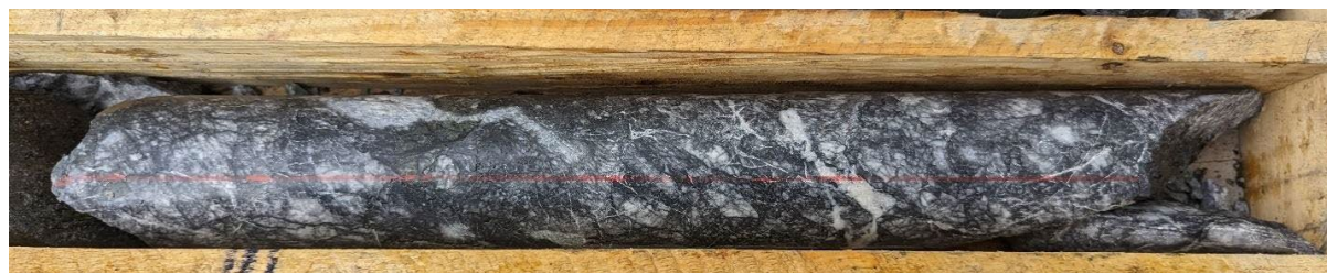
(Photo 6) Drill hole SB14 05. Mineralized breccia of gold bearing orogenic quartz vein returning 0.65 gpt Au, >10,000ppm (>1%) Zn, 0.12% Cu, 2.51 gpt Ag over 0.80* meters (From 153.7m to 154.5m), part of a larger interval from 153.7 to 155.7m (See Table 1)
