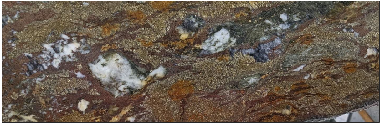
Photo 2. Semi-massive pyrite replaces almost 50% of the rock, clearly following high-strain zones within these deformation zones (shear zones), and dark red/brown sphalerite starts replacing (10%) the pyrite from the edges and at clast boundaries in pressure shadow zones. (D13-01A detail from interval 83.5m to 84.3m). For assay results refer to Table 3.
