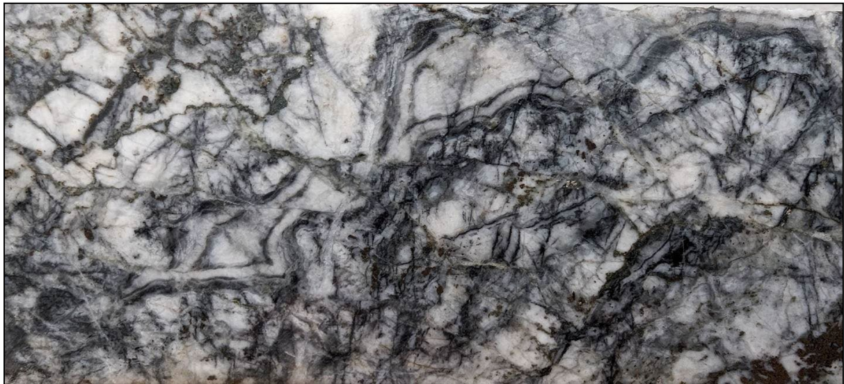
Photo 1. Complex banded, crustiform, breccia textures in gold bearing quartz vein. D13-01A (31.66 gpt Au from 114.75 to 115.7). For assay results refer to Table 3.
